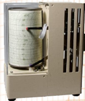
Hygromograph (image from Oakton Instruments) and graph paper.
